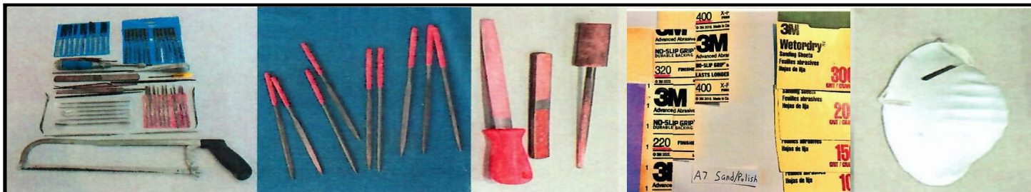
Use tools such as hand saws, files, awls, various grades of emory cloth and a face mask for dust protection.
